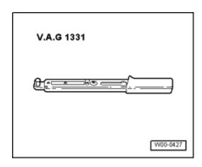
■ Torque wrench (5 to 50 Nm) V.A.G 1331
